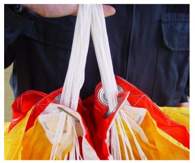
We find the A group of lines on one side of the canopy. We should hold the canopy in front of ourselves, as we have it now, A lines form front part of line groups going through the front passages of the slider (part, which is the closest to us).
