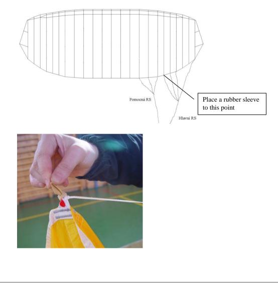
Fold the trailing edge into S-folds in a similar way to stabilizers. Stretch the steering lines and auxiliary steering lines and turn the excess auxiliary steering lines twice around the forefinger and middle finger of left or right hand, and put the resulting twist into a rubber sleeve.
