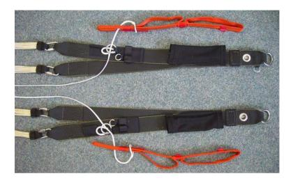
The auxiliary equipment steering loops are placed nearer the centre. The placement and connection is shown in the picture.
