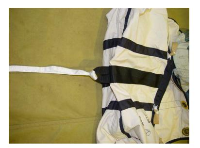
**2. The deployment bag attachment to the main canopy.** Check if the eye at the attachment point of the main canopy is intact and not damaged and if the main canopy is not damaged near the deployment bag attachment point. Then check a fast connection between the bag and main canopy.
