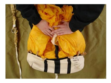
Hold the canopy with your free hand at the place where the main canopy container is connected and fold it back over the enfolding arm towards the packing pad. Smooth the container and insert a left or right part of the first canopy fold into the container as shown in the picture. Then repeat this step on the opposite side.
