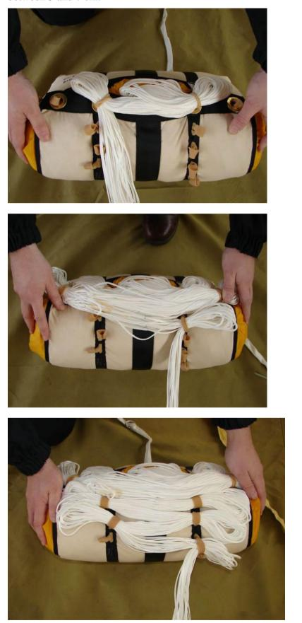
Close the deployment bag with a suspension line bundle. Put the remaining suspension line length into rubber sleeves so that the length of single loop is between 5 and 7 cm.
