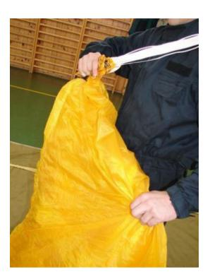
Insert the rolled-up trailing edge part into the parachute centre (see the picture).
