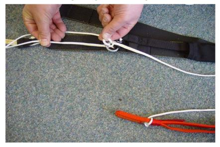
Interlaced brake loop fix by reinforced part of the main canopy steering loops RP-009 TC-1.
