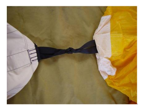
**3. Outside canopy fabric.** Stretch the canopy with upper canopy fabric upwards and check the upper fabric. Concentrate on tears, stains and damaged seams. Check the fabric strength in such a way that you hold a part of the fabric in each hand and with not a very strong pull, try to tear the canopy.
