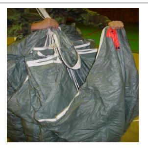
Roll the canopy trailing edge evenly around the stowed canopy and align the left and right sides in such a manner that the seams and trailing edge trims are placed against each other.
