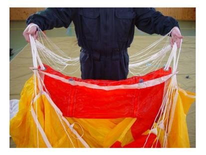
After the lines are checked, connect suspension lines into one joint bundle. Now, place the parachute lines on a random shoulder in such a manner that the stops on the main parachute canopy are at the same height. Use one hand to list individual canopy cells leading parachute edge in an order form A-1 to A-10.
