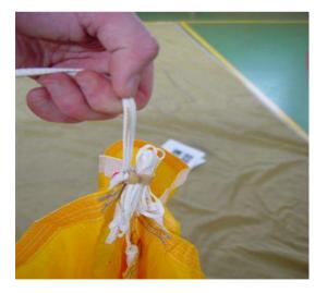
The next step is to check if the stabilizers and their slider stops are in the proper position outside the suspension lines. If the stabilizer (or its slider stop) lies under the line, the canopy could possibly become damaged. The canopy stowed in this way should look like in the following picture.
