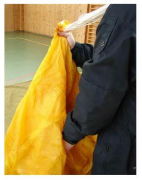
Put your free hand under the canopy carefully. Swing slightly the canopy so that the lines remain stretched and place it slowly on the pad in such a way that the canopy remains evenly divided into halves.
